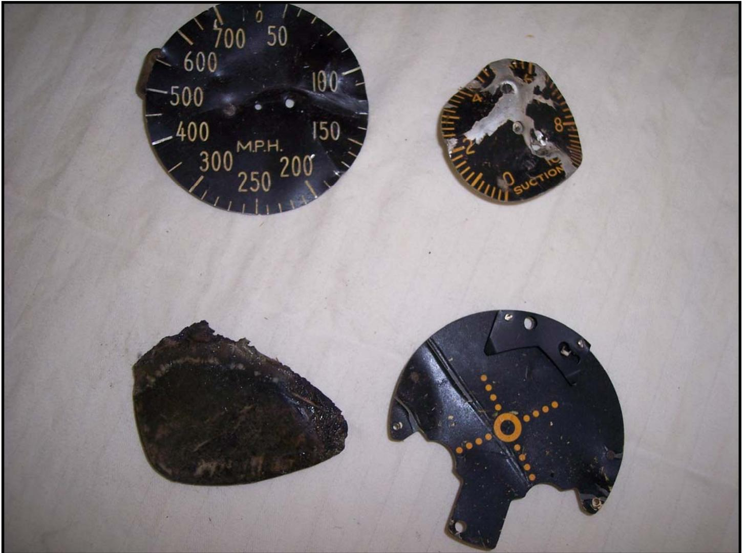
Three of these are parts of instrument gages. The item on the left, bottom, is the burnt lens of a pair of sun glasses.
